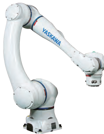
Collaborative robot MOTOMAN-HC20DTP
